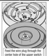
Note: Remove the pre-installed light kit assembly screw and red flag from the light kit assembly. Save the screw. It will be needed for installation
