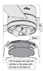
Attach the globe by lifting and turning clockwise one third of a full turn of the glass until it stops.
