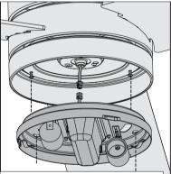
Connect the plugs from the upper and lower switch housings. Make sure to line up the colored markings on the connectors. Align the keyhole slots in the light kit housing with the two screws. Make sure all the wires from the fan and the light kit are snug inside the center of the light kit, not pinched in between the upper switch housing and the light kit or hanging out of the sides.
