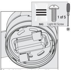
Turn the light kit counterclockwise until the switch housing screws are firmly situated in the narrow end of the keyhole slots. Install the third screw and tighten all three screws securely.
