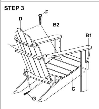
Attach backrest (D) onto the assembly from step 2. Secure the backrest (D) to armrest (B1&B2) with 1" bolts (F).
