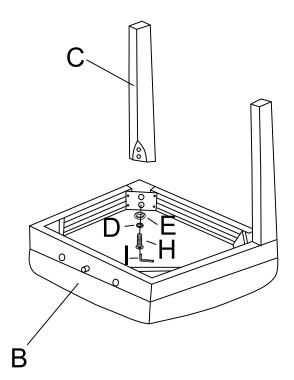
Take the Allen Wrench, and turn the bolts until the legs are secure.
