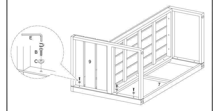
Attach right leg (9) to back frame (7) using short bolts (B) and washers (C) . Tighten short bolts (B) with wrench (E). Hands tighten all bolts only and not tighten completely.
