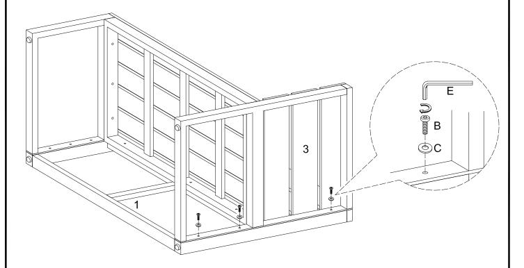
Attach left leg (3) to back frame (1) using short bolts (B) and washers (C) . Tighten short bolts (B) with wrench (E). Hands tighten all bolts only and not tighten completely.
