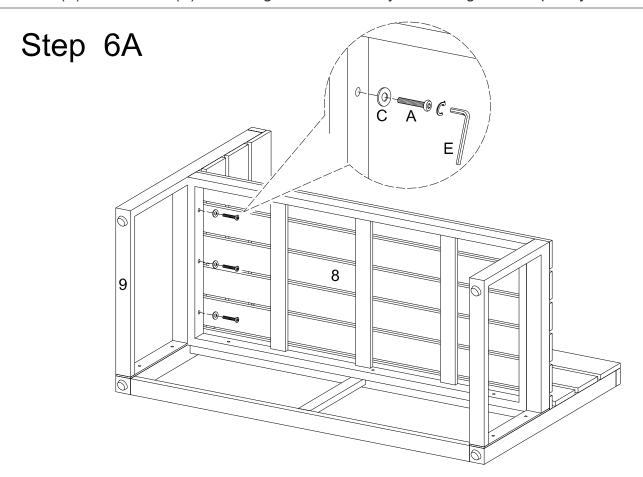
Attach seat frame (8) to right leg (9) using long bolts (A) and washers (C) . Tighten long bolts (A) with wrench (E). Hands tighten all bolts only and not tighten completely.
