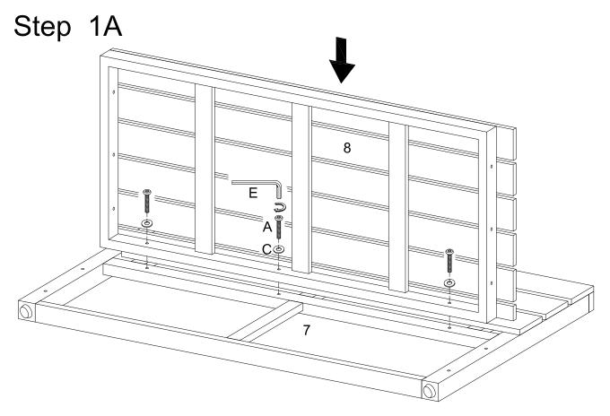
Attach seat frame (8) to back frame (7) using long bolts (A) and washers (C) . Tighten long bolts (A) with wrench (E). Hands tighten all bolts only and not tighten completely.
