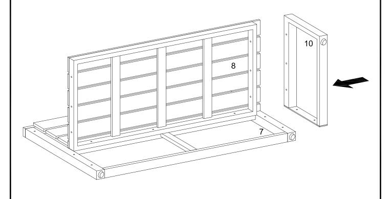
Attach left leg (10) to seat frame (8) using bolts as guides.
