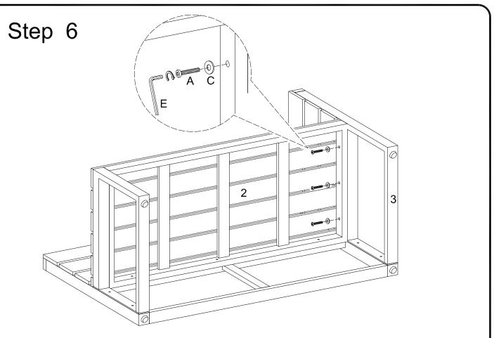
Attach seat frame (2) to left leg (3) using long bolts (A) and washers (C) . Tighten long bolts (A) with wrench (E). Hands tighten all bolts only and not tighten completely.
