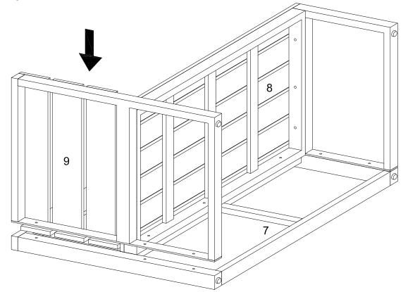
Attach right leg (9) to back frame (7) using bolts as guides.
