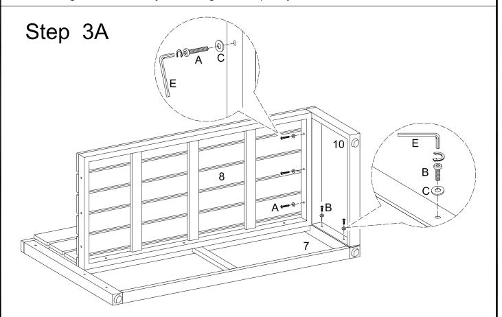
Attach seat frame (8) to left leg (10) using long bolts (A) and washers (C). Attach left leg (10) to back frame (7) using short bolts (B) and washers (C). Tighten all bolts with wrench (E). Hands tighten all bolts only and not tighten completely.
