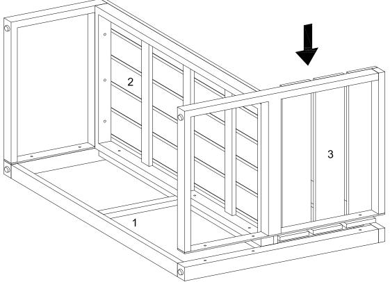
Attach left leg (3) to back frame (1) using bolts as guides.
