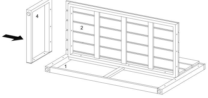
Attach right leg (4) to seat frame (2) using bolts as guides.
