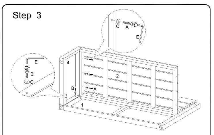
Attach seat frame (2) to right leg (4) using long bolts (A) and washers (C). Attach right leg (4) to back frame (1) using short bolts (B) and washers (C). Tighten all bolts with wrench (E). Hands tighten all bolts only and not tighten completely.
