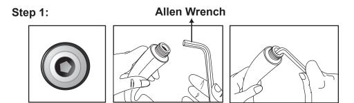
Insert the Allen Wrench Into the bottom of the handheld shower.
