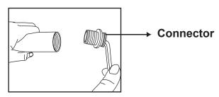
Remove the Connector by turning the Allen Wrench counter-clockwise.
