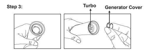
Remove the Generator Cover. Clean the Turbo and turn the Turbo Step 4: a couple turns.
