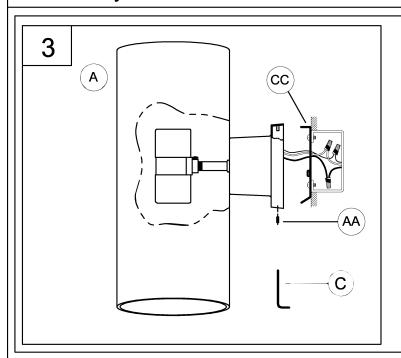
3. Attach fixture (A) to mounting plate (CC). Use set screw (AA) and allen wrench (C) to secure tightly.
