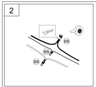
2. Strip 3/8" of insulation from the electrical wire ends. Using wire nuts (BB), connect white fixture wire to the white supply wire from the outlet box; connect the black fixture wire to the black supply wire.
