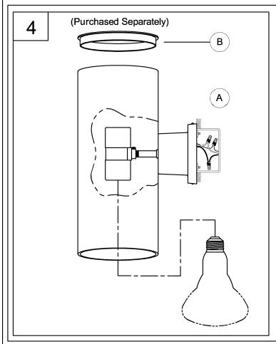
4. Screw two lamps (not included) into fixture socket. Use 75-watt MAX (65-watt MAX for P5713) incandescent medium base lamp, R30 or PAR30.
