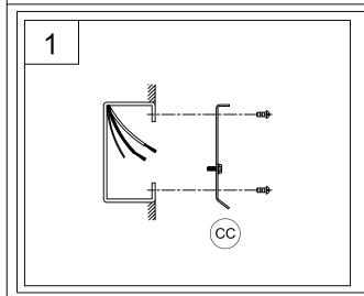
1. Attach mounting plate (CC) to outlet box using the mounting screws supplied with the outlet box (not included).
