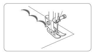
For a delicate appearance on fabric such as chiffon, use a single layer with a tear-away backing, if necessary.
