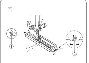
1 With the buttonhole foot raised, hook the filler cord on the spur at the back of the foot. Bring the ends toward you under the foot, clearing the front end.
