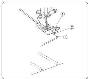
Fold a fabric wrong side together and Lower the needle into the fabric 0.1 - 0.2 cm inside the folded edge.
