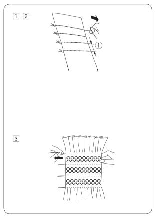
1 Choose a soft and lightweight fabric such as batiste, gingham or challis. Cut the fabric three times wider than the project width. Increase the stitch length to "4" and loosen thread tension to "1". Sew rows of straight stitches 3/8" (1 cm) apart across the area to be smocked.
