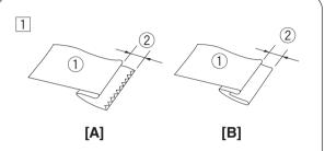
1 On heavy weight fabrics that ravel, the raw edge should be overcast first.
