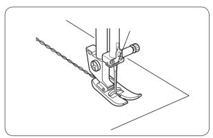
The pattern is sewn with two stitches forward and one stitch backward, forming a seam that does not rip easily.
