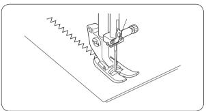
Simple zigzag stitching is widely used for overcasting, sewing on buttons etc.
