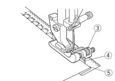
3 Turn the screw to align the guide on the foot with the folded edge so that the needle just pierces the fold.
