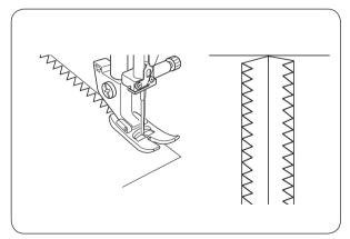
The zigzag stitch is used on the seam allowance to prevent fabric from fraying at raw edges.
