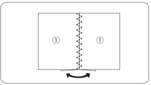
Place two layers of the fabric with the right side together. Seam along the edges with the straight stitch.
