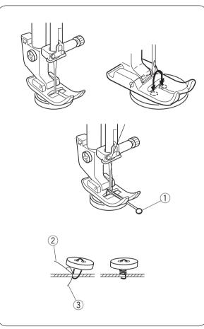
Unthread the needle. Adjust the stitch width to match it with the span of the holes in the button. Turn the handwheel to check if the needle enters into each hole in the button.
