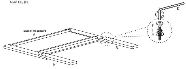
Attach Side Rail (E) to Headboard (A) and Footboard (C) by inserting JCBB Bolts (G) loosely into provided holes, then hook Side Rail brackets on as shown. Tighten all bolts using Allen Key (L).
