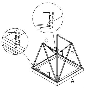
Step 2: Put the bottom shelf part (D) on top of the (B&C) Metal legs and locate the threaded inserts into the holes in bottom panel and then fasten the bolts.
