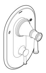
**BELFIELD™ POSI-TEMP®** with Built-In 3 Function **Transfer Valve Trim**
