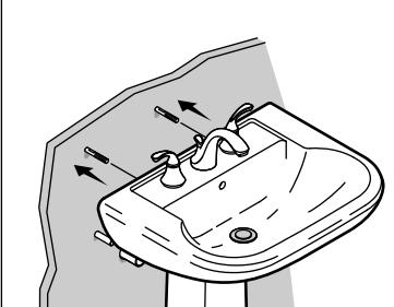
**16** Level and secure the sink using cap nuts and washers. **Do not overtighten!**
