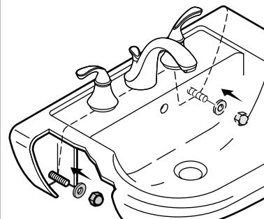
**17** Complete the faucet and drain connections. Run water and check for leaks.
