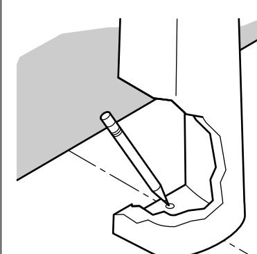
**11** Move the sink and pedestal aside. Drill 1/4" holes at the three marked locations.
