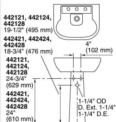
**2** The supply stops, when fully open, should not contact the pedestal.
