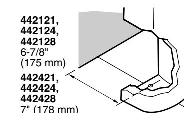
**7** Set the sink on the pedestal and against the wall. If necessary, adjust the pedestal.
