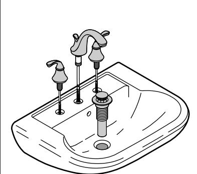
**15** Position the sink on the pedestal so the hanger bolts extend through the anchoring holes.
