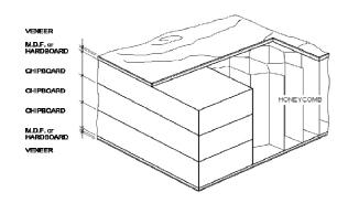
All 1.6 cm thick components are made of regular chipboard or particle board. Thicker components are made of sandwich construction with a solid chipboard frame. Additional cross bars are used for larger elements.
