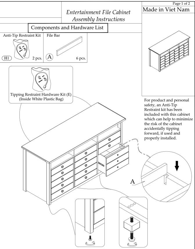
There are levelers underneath the Console which can be adjusted to compensate for uneven flooring. If the furniture wobbles, determine which corner does not touch the floor correctly. With two people follow these steps:
