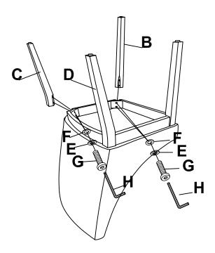
Stand chair up on an even surface and check that it is balanced. If there is a slight wobble, apply downward pressure in the corner where a leg isuneven. Keeping pressure in that corner, tighten all bolts. If balanced, apply downward pressure evenly in the center and tighten all bolts. Do not over-tighten beyond hole depth.
