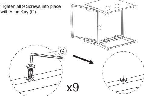
**NOTE**:IF ANY SCREW HOLES CANNOT BE ALIGNED, LOOSEN ALL THE SCREWS AND GO BACK STEP 1 AND RESTART ASSEMBLY.
