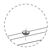
NOTE:IF ANY SCREW HOLES CANNOT BE ALIGNED, LOOSEN ALL THE SCREWS AND GO BACK STEP 1 AND RESTART ASSEMBLY.
