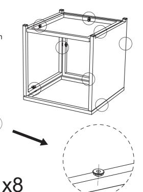
NOTE:IF ANY SCREW HOLES CANNOT BE ALIGNED, LOOSEN ALL THE SCREWS AND GO BACK STEP 1 AND RESTART ASSEMBLY.
