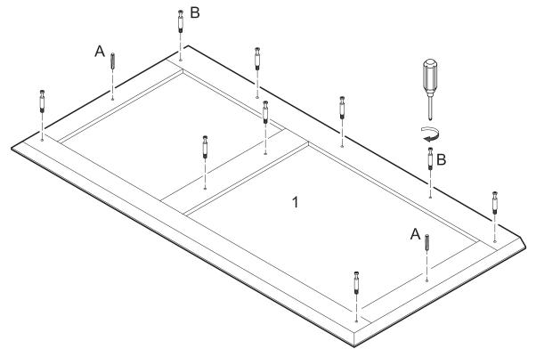
Insert dowels (A) into desk top (1). Screw cam bolts (B) into desk top (1) with a screwdriver.
