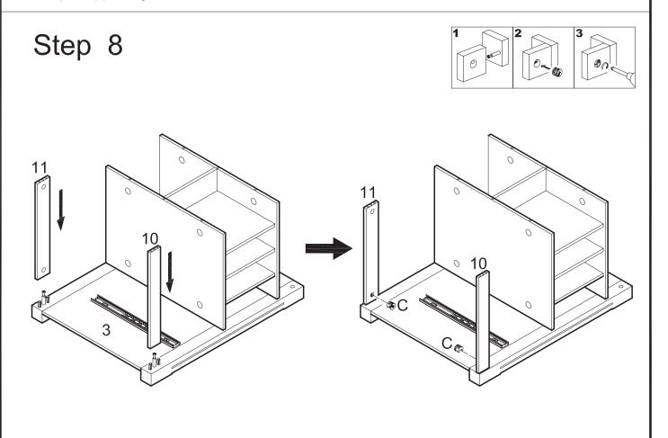
Fit slats (10,11) onto panel (3) using cam bolts and dowels as guides. Insert cam locks (C) into slats (10,11) and tighten with a screwdriver.
