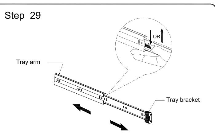
For disassemble drawer tray ,by sliding the tray arm and the tray bracket out. Press and tick the small lever on the tray bracket and carefully pull the two pieces apart.
