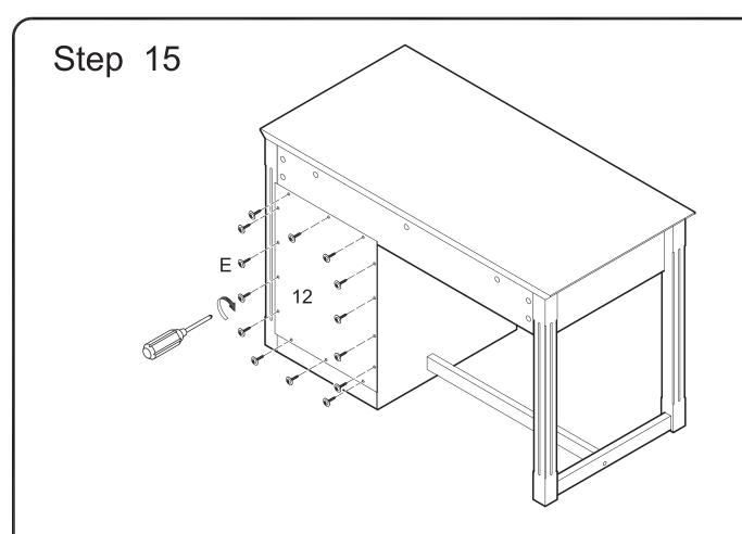
Attach back panel (12) to desk frame using screws (E). Tighten screws (E) with a screwdriver.
