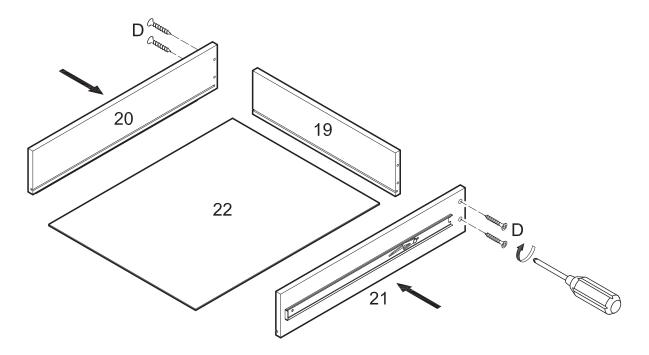
Attach drawer sides (20,21) to drawer back (19) using screws (D). Carefully slide drawer bottom (22) into place along the grooves of the drawer assembly.
