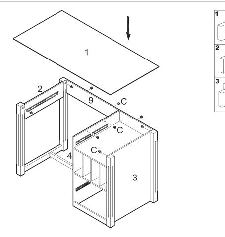
Insert cam locks (C) into panels (2,3,4) and slat (9). Fit desk top (1) into place using cam bolts and dowels as guides. Tighten cam locks (C) with a screwdriver to secure desk top (1).
