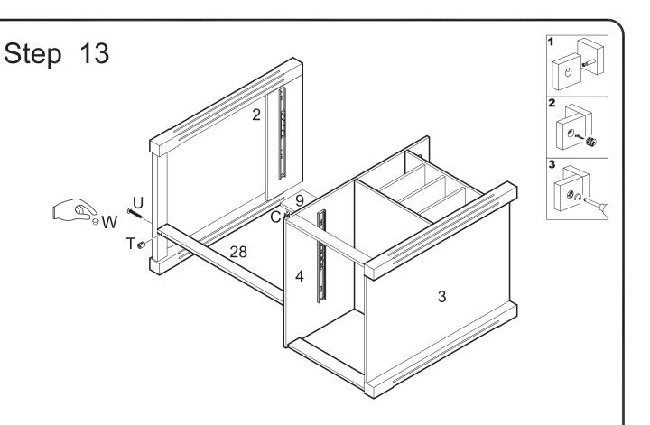
Insert cam locks (C) into slat (9) and tighten with a screwdriver. *Note that two cam locks (C) will be inserted into slat (9).* Insert barrel nut (T) into slat (28). Secure slat (28) to panel (2) using bolt (U). *Note that bolt (U) will screw directly into barrel nut (T).* Cover bolt (U) with cap (W).
