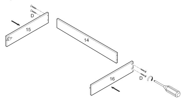
Attach drawer sides (15,16) to drawer back (14) using screws (D). *Insure that the drawer locks are on the interior of the drawer assembly.* Tighten screws (D) with a screwdriver.
