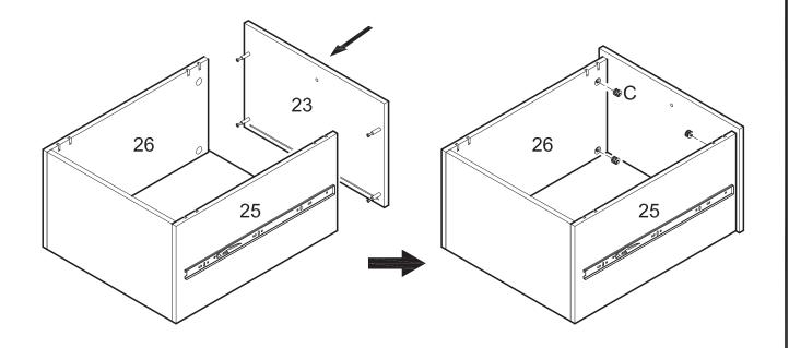
Fit drawer front (23) onto drawer sides (25,26) using cam bolts as guides. Insert cam locks (C) into drawer sides (25,26) and tighten with a screwdriver. *Note that two cam locks will be inserted into each drawer side*.
