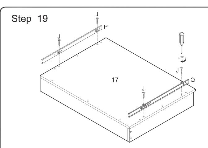
Attach left drawer track (P) and right drawer track (Q) to drawer bottom (17) as shown above using screws (J). Tighten screws (J) with a screwdriver.
