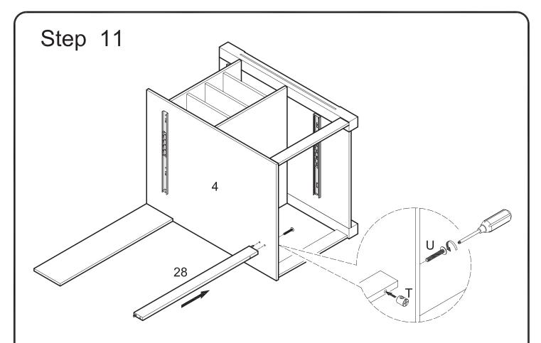
Fit slat (28) onto panel (4) using dowel as a guide. Insert barrel nut (T) into slat (28). Secure slat (28) to panel (4) using bolt (U). Note that bolt (U) will screw directly into barrel nut (T).
