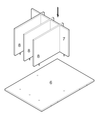
Fit divider panels (7,8) onto panel (6) using dowels as guides.
