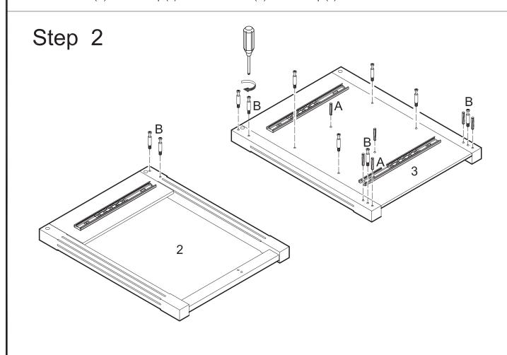
Insert dowels (A) into panel (3). Screw cam bolts (B) into panels (2,3) with a screwdriver.
