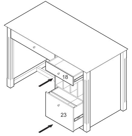
Carefully slide the remaining drawers into place. Note that you will need to align the metal tracks of the drawers with those on the desk to slide the drawers into place.
