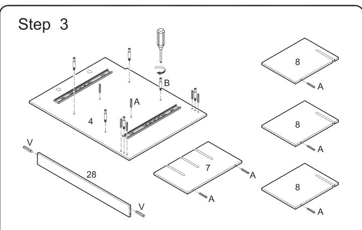
Insert dowels (A) into panel (4) and divider panels (7,8). Screw cam bolts (B) into panel (4) with a screwdriver. Insert dowels (V) into slat (28).
