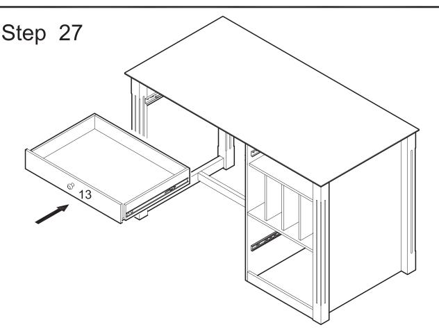
Carefully slide the drawer into the desk assembly. Note that you will need to align the metal tracks of the drawer with those on the desk to slide the drawer into place.
