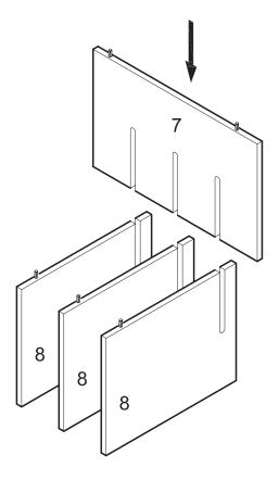
Carefully slide divider panel (7) into place along the notches of divider panels (8).
