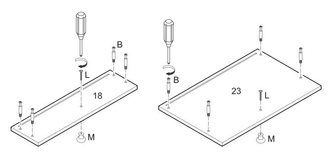
Screw cam bolts (B) into drawer fronts (18,23) with a screwdriver. Attach knobs (M) to drawer fronts (18,23) using bolts (L).
