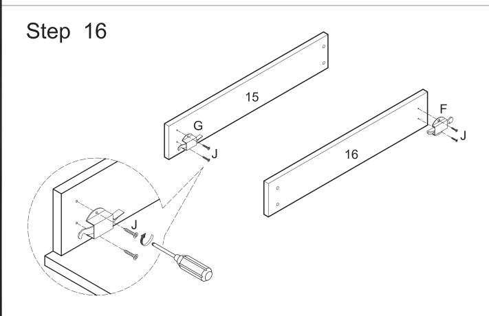
Attach left drawer lock (G) to drawer side (15) using screws (J). Attach right drawer lock (F) to drawer side (16) using screws (J) . Tighten all screws (J) with a screwdriver.
