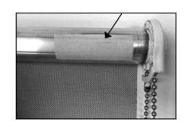
The chain connector on the back of the chain will prevent the roller shade from being raised past its limit. In order to prevent the shade from being lowered past the ordered length, we have provided plastic stop balls that are easily snapped onto the chain. (Note: Additional material has been added to the ordered length to prevent exposure of the roller tube).
