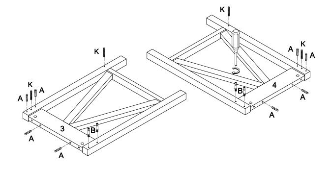
Insert wooden dowel (A) and secure cam bolt (B,K) to side frame (3,4).
