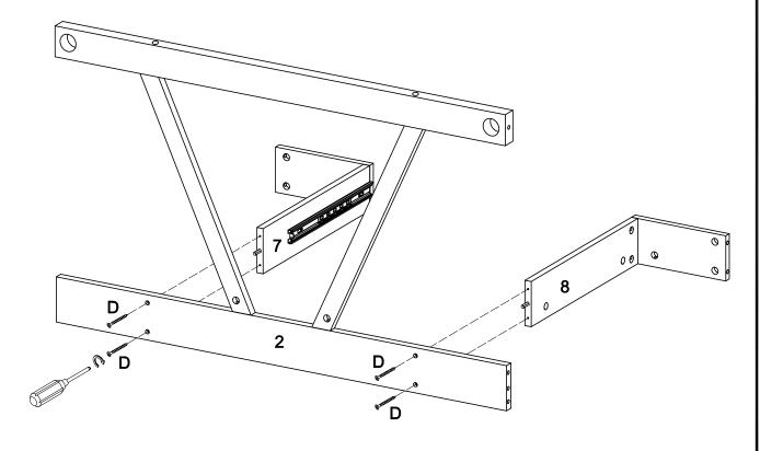
Insert side panel (7,8) into back panel (2), then secure it with screw (D).
