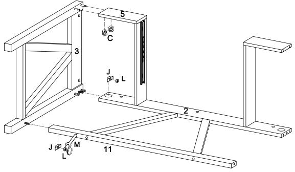
Insert side frame (3) into back panel (2) and parts (5,11), then insert and secure cam lock (C) to parts (5), and use wrench (M) to secure back panel (2) and part (11) with half moon washer (J) and nut (L) to lock them.
