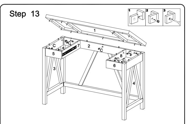
Insert top panel (1) into desk frame, then insert and secure cam lock (C) to back panel (2), side frame (3,4), side panel (7,8), and parts (5,6) to lock it.
