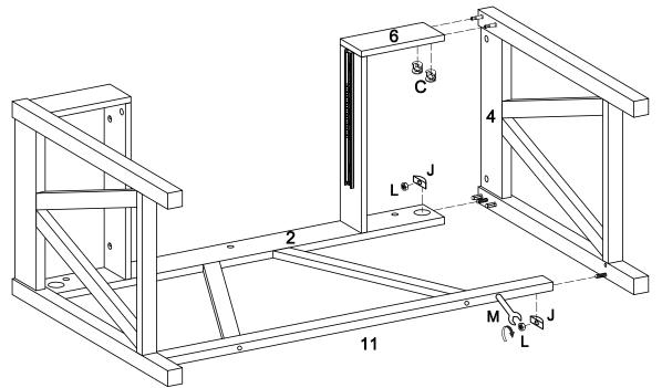
Insert side frame (4) into back panel (2) and parts (6,11), then insert and secure cam lock (C) to parts (6), and use wrench (M) to secure back panel (2) and parts (11) with half moon washer (J) and nut (L) to lock them.
