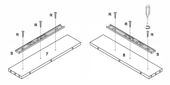
Secure drawer slider arms (S) to side panels (7,8) with screw (R).
