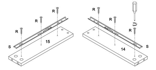
Secure slider brackets (S) to drawer side panel (14,15) with screw (R).
