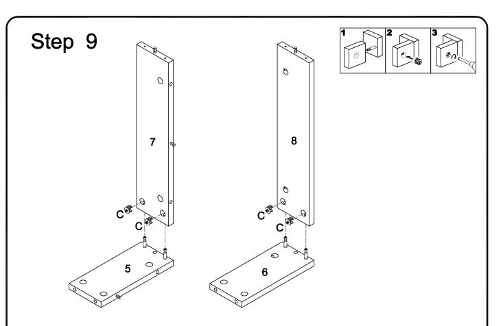
Insert parts (5,6) into side panel (7,8), then insert and secure cam lock (C) to side panel (7,8) to lock it.
