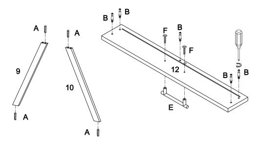
Insert wooden dowel (A) to parts (9,10). Secure cam bolt (B) to drawer front panel (12), then secure handle (E) with bolt (F).
