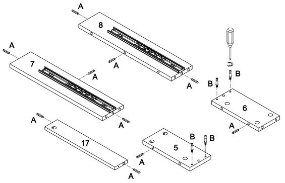
Insert wooden dowel (A) to side panel (7,8) and parts (5,6,17). Secure cam bolt (B) to parts (5,6).
