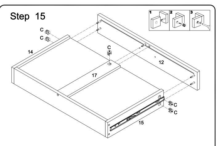
Insert drawer front panel (12) into drawer side panel (14,15) and parts (17), then insert and secure cam lock (C) to drawer side panel (14,15) and parts (17) to lock it.
