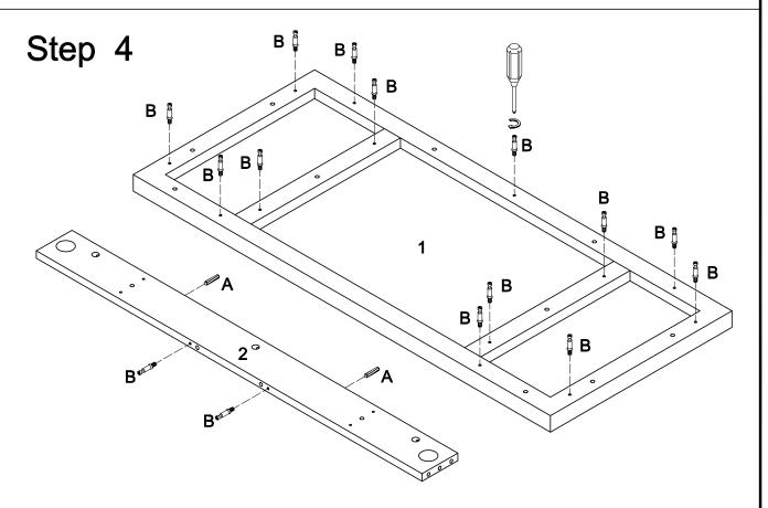
Secure cam bolt (B) to top panel (1). Insert wooden dowel (A) and secure cam bolt (B) to back panel (2).
