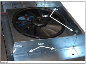
Semove and set aside the 4 front screws retaining the bent plate to the hood.
