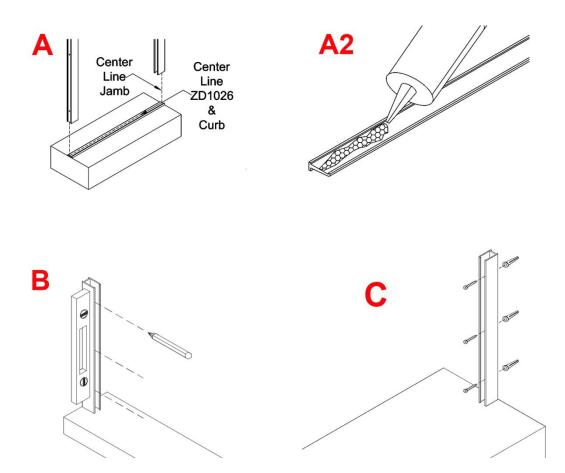
the hinge side wall jamb. Do not fasten the door at this point (D).
