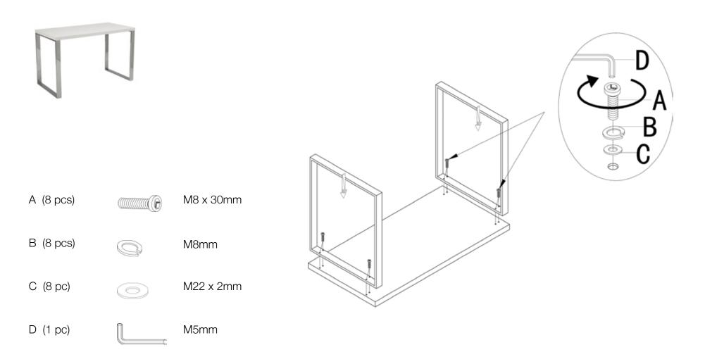
During assembly, hand tighten screws only. When all screws are in place, then tighten completely.
