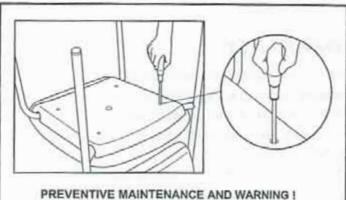
From time to time, check to make sure screws are securely tightened. O Holes on PP shell are for convenient checking.
