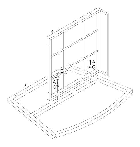
Attach part (4) to part (2) using bolt (A) and washer (C) with hex key (E).
