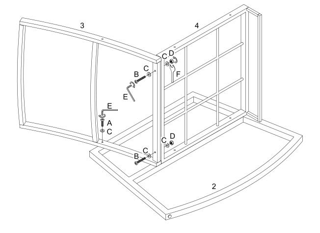
Attach part (3) to part (2, 4) using bolt (A, B), nut (D) and washer (C) with hex key (E) per diagram.
