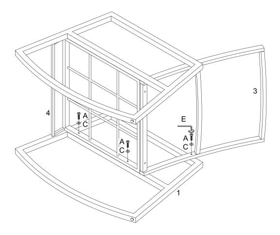
Attach part (3, 4) to part (1) using bolt (A) and washer (C) with hex key (E) as per diagram.
