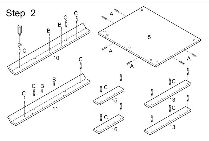
Insert the cam bolts (C) to the front panel (10,11,13,15,16). Insert the wooden dowel (B) to the front panel (10)(11) and wooden dowel (A) to middle panel (5).
