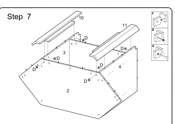
Attach the front panel (10)(11) to the side panel (3)(4) and secure it by using cam locks (D).
