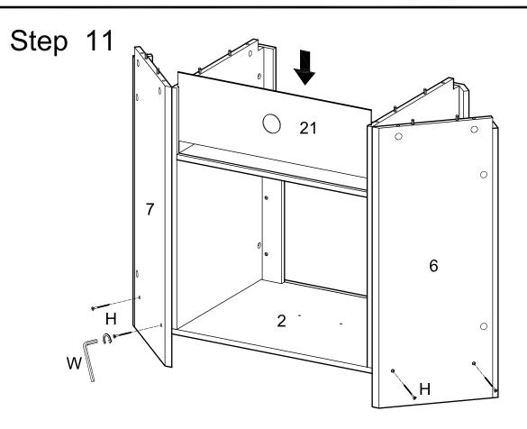
Attach the side panel (6)(7) to the bottom panel (2) and secure it by using screw (H) and wrench (W). Insert the back panel (21) into the slot of side panel (6)(7).
