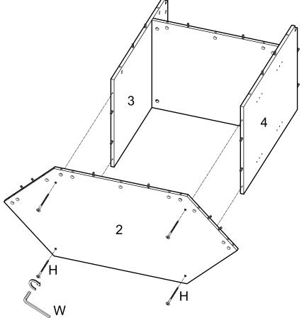
Attach the bottom panel (2) to the side panel (3)(4) and secure it with screw (H) and wrench (W).
