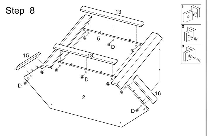
Attach the front panel (13)(15)(16) to the bottom panel (2) and middle panel (5) by using cam locks (D).
