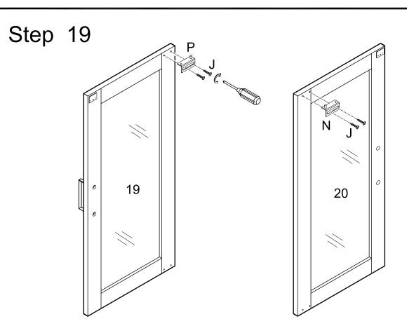
Attach the door hinge (P)(N) to the glass doors (19)(20) and secure it by using screw (J).
