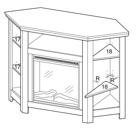
Insert the shelf support pin (R) into the stand and place the shelf (17)(18) on top.
