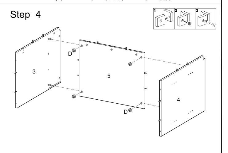
Attach the side panel (3)(4) to the bottom panel (5) and secure it with the cam locks (D).
