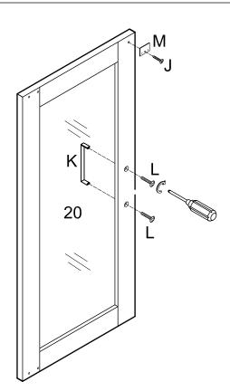
Attach the metal piece (M) to the glass doors (19)(20) and secure it by using screw (J). Attach the door knob (K) to the glass doors (19)(20) and secure it by using screw (L).
