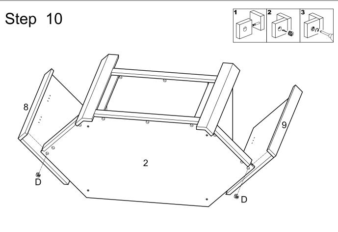
Attach the side panel (8)(9) to the bottom panel (2) and secure it by using cam locks (D).
