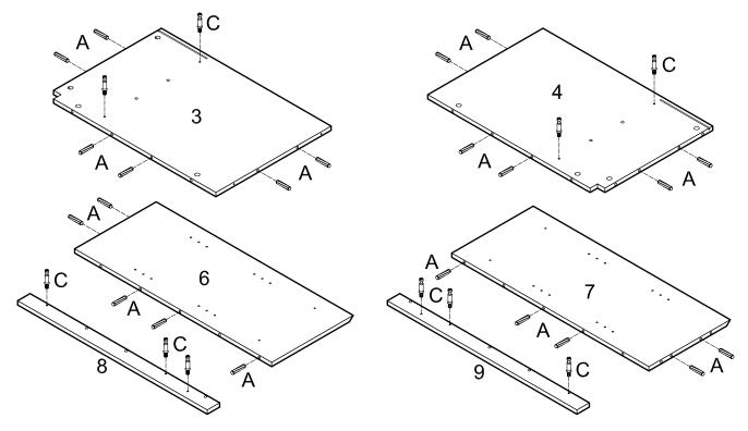
Insert the wooden dowel (A) into the side panel (3,4,6,7). Insert the cam bolts (C) into the side panel (3,4,6,7) and front panel (8)(9).
