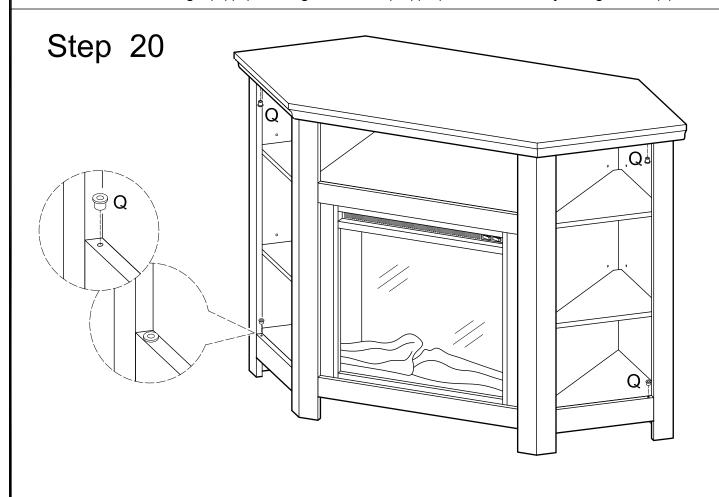
Insert the plastic pivot (Q) as shown as the diagram.
