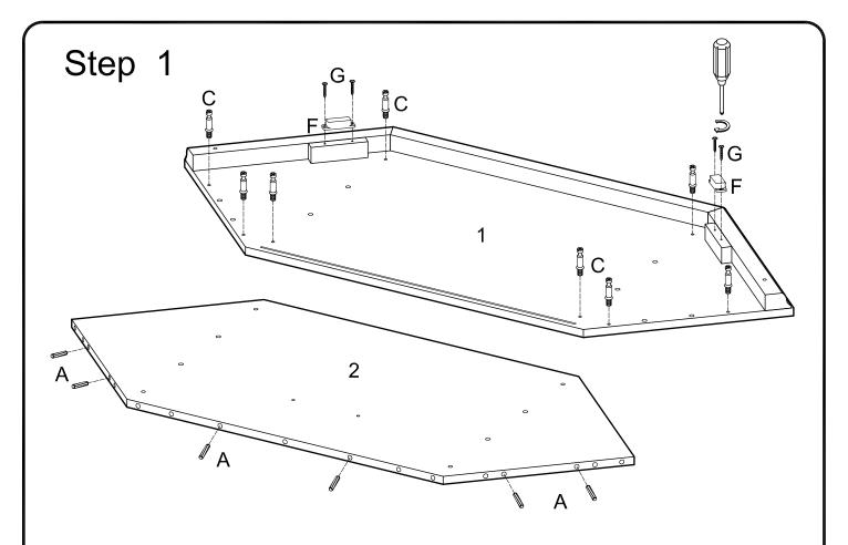
Insert the cam bolts (C) and door stopper (F) into the top panel (1) by using screws (G). Insert the wooden dowel (A) to the bottom panel (2).
