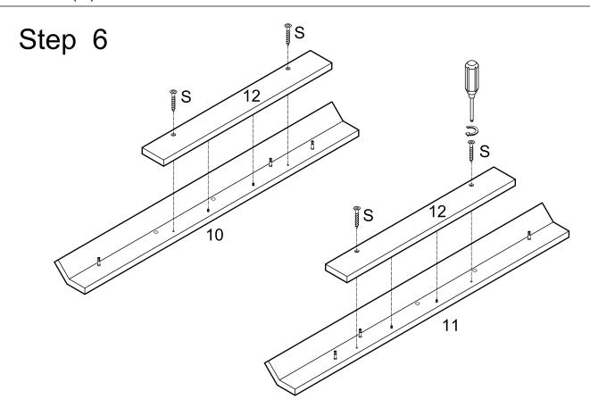
Attach the support slats (12) to the front panel (10)(11) and secure it by using screw (S).
