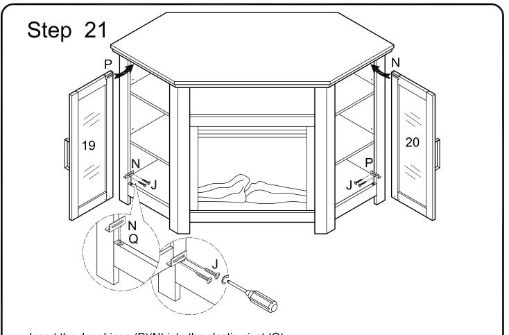
Insert the door hinge (P)(N) into the plastic pivot (Q). Insert the doors (19)(20) as shown in diagram and secure it with screw (J).
