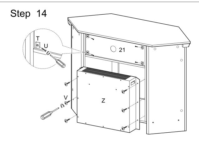
Secure the back panel (21) by using the plastic wedge (T) and screw (U). Put the fireplace insert (Z) carefully into the stand and secure it by using screw (V).
