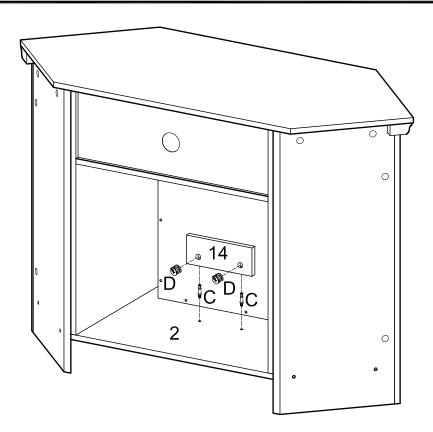
Insert the cam bolts (C) to the bottom panel (2) and attach the support panel (14) to the bottom panel (2) by using cam locks (D) to secure it.
