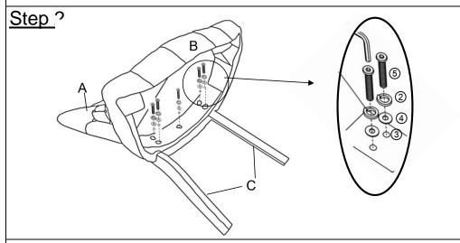
Place the Back with Legs(B) on a clean, non-marring surface. Align the mounting positions on the Seat(A) to the mountings on the Back with Legs(B).
