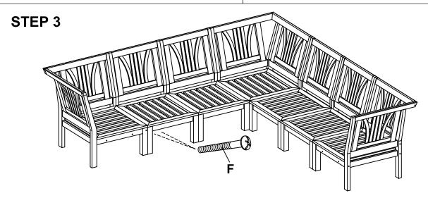
Joint all the corner chairs and other chairs as shown. Secure using 2" bolts from underneath of seat. Make sure all parts are correctly connected and tighten all bolts using screwdriver.
