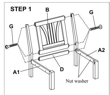
Attach right and left side frame (A1 & A2) into back support (B) and apron (D). Secure using 1 1/2" bolts (G) as shown.
