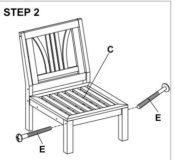
Next, attach the seat (C) into pre-assembled side frames and secure using 2 1/4" bolts (E) as shown. Tighten all bolts completely using screwdriver.
