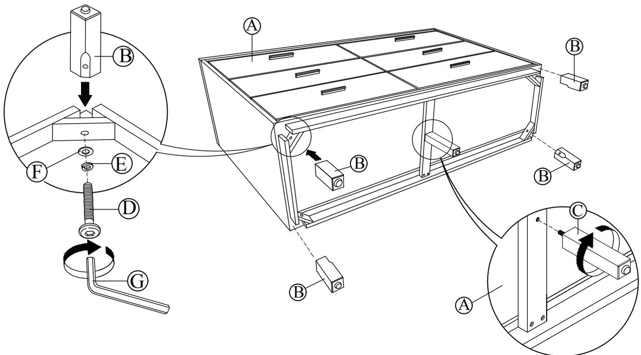
Insert Leg (B) at position as shown and tighten with JCBC Screw (D), Spring Washer (E) & Flat Washer (F) by using Allen key (G). Rotate and tighten Center Support Leg (C) to center of the bottom Dresser.
