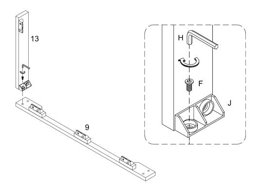
Attach plastic wedge (J) to part (9) using bolt (F) with Hex key (H).
