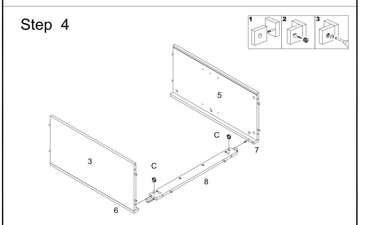
Attach part (3,6,5,7) to part (8), then insert and secure cam lock(C) to part (8) to lock
