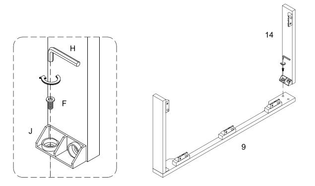
Attach plastic wedge (J) to part (9) using bolt (F) with Hex key (H).
