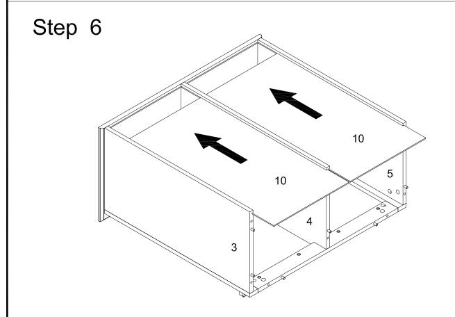
Slide back panel (10) into grooves as per diagram.
