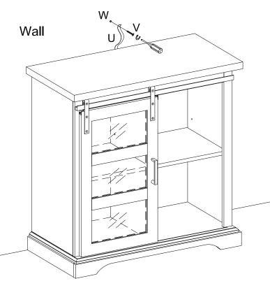
Secure product to wall with screw (V), through Plastic strap(U) by using screwdriver
