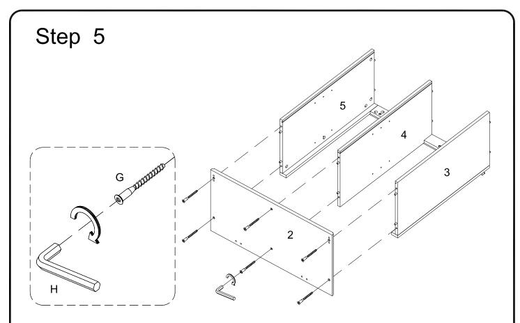
Attach part (2) to part (3,4,5) using screw (G) with hex key (H). Note: Groove for back panel should be aligned.
