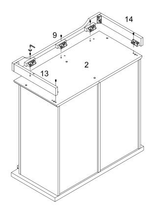
Attach part (9,14,13)to part (2) using plastic wedge( J) bolt (F) with hex key (H).
