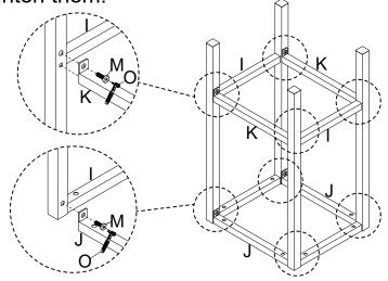
Take the Ratchet Tool, and turn the bolts until the legs are secure. DO NOT TIGHTEN COMPLETELY. Stop when you feel you are adding force to tighten the bolts.
