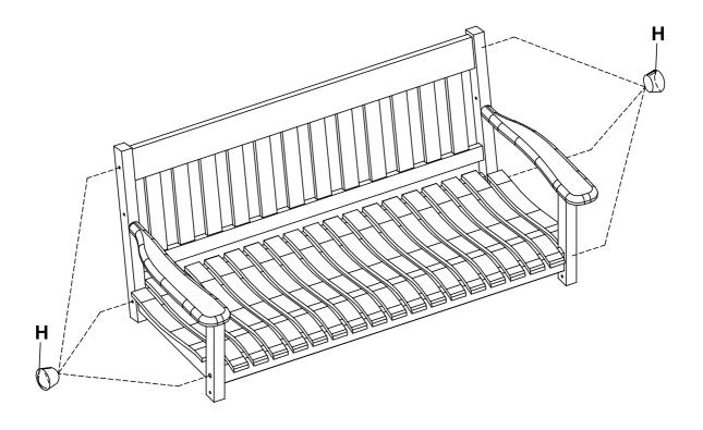
Tighten all bolts completely using screwdriver and tipping in the wooden caps (H). to cover bolts head using rubber mallet.
