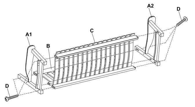
Install on level ground. Attach the back support (B) and seat (C) into right and left side frames (A1 & A2). Secure using 1 1/4" bolts (D). as shown.
