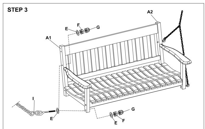
Secure the hanger bolts with chain (I) into predrilled holes of right side frame (A1), using washers (E), nuts (F) and head nuts (G) as shown.
