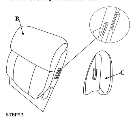
Insert both back rests and console back rest to the seat frame.
