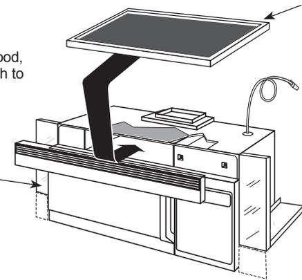
Filter Kit JX81L-Recirculating Charcoal Filter Kit To be used when the Spacemaker microwave oven cannot be vented to the outside.
