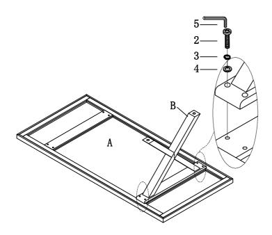
Lock a side of cross bar(C) to leg frame(B) by using flat washer(4), lock washer(3) ,bolt-large(1), allen key(5) and wooden dowel(6).
