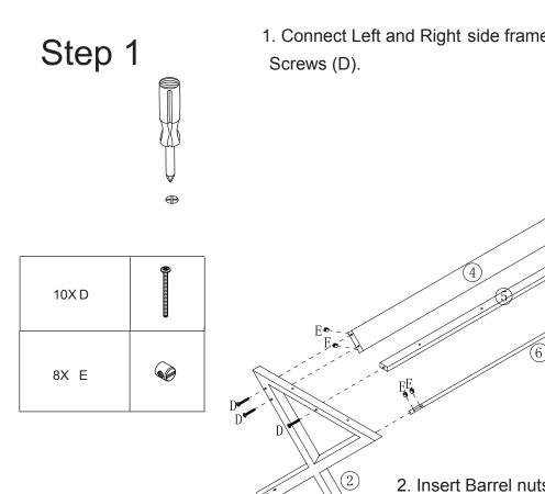
1. Connect Left and Right side frames ② and ③ to Support bar ⑤ using
