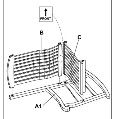
Attach back support (B) and seat (C) on to right side frame holes (A1).
