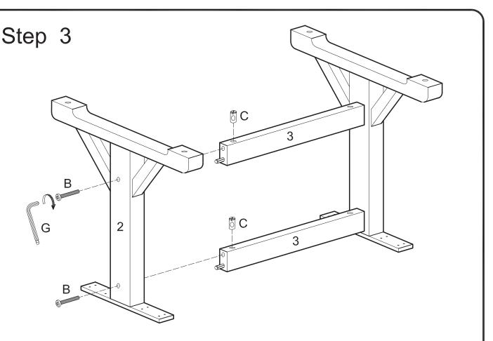
Insert nuts (C) into opposite ends of crossbars (3). Attach crossbars (3) to second leg piece (2) using bolts (B). Tighten bolts (B) with wrench (G). Bolts (B) will screw directly into nuts (C).
