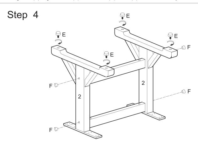
Screw feet (E) into leg pieces (2). Insert wood buttons (F) into leg pieces (2).
