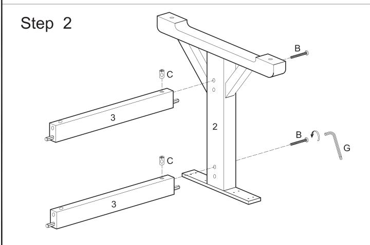
Insert nuts (C) into crossbars (3). Attach crossbars (3) to leg piece (2) using bolts (B). Tighten bolts (B) with wrench (G). Bolts (B) will screw directly into nuts (C).
