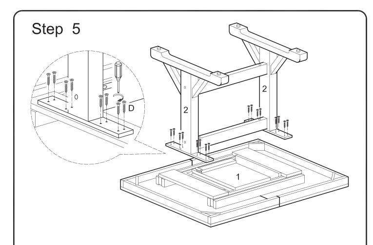
Attach leg pieces (2) to table top (1) using screws (D). Tighten all screws (D) with a screwdriver.
