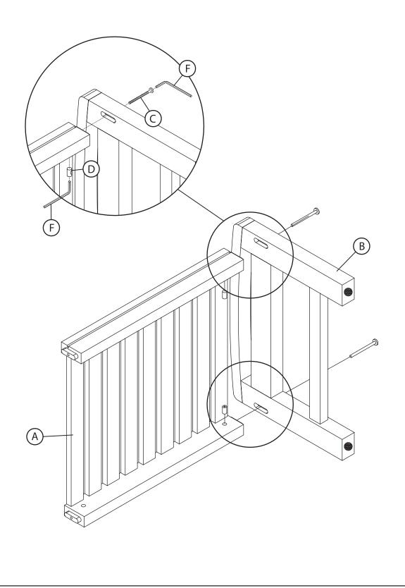
**ATTACH REMAINING LEG FRAME TO BASE -** Repeat the process in the same order from step one on the opposite side of the frame.
