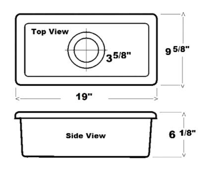
Dimensions of fixture are nominal and may vary within the range of tolerances established by ANSI Standard A112.19.9. Dimensions and specifications subject to change without notice.
