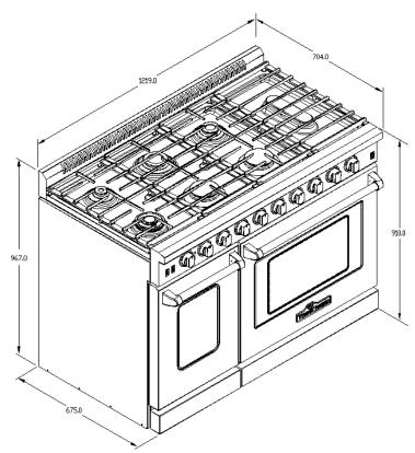
The maximum depth of cabinets installed above cooking tops be 13 in (330mm) or a great specified by the manufactures as tested by the certification agency.
