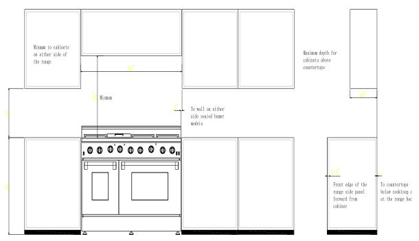
The bottom of the hood should be 30" min. to 36" above the counter top. This would typically result in the bottom of the hood being 66" to 72" above the floor. These dimensions provide safe and efficient operation of the hood.
