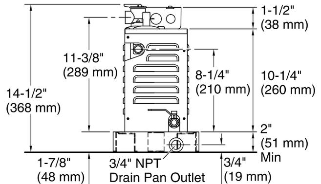
Minimum required access panel is 24" (610 mm) L x 15" (381 mm) H.
