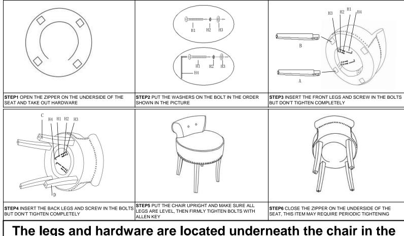
The legs and hardware are located underneath the chair in the zipper compartment.
