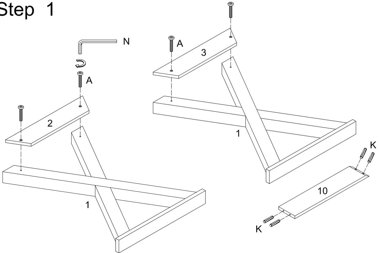
Attach Side Panel (2) & (3) with Screws (A) to the Legs (1), Insert the Wooden Dowels (K) into the Support Bar (10).
