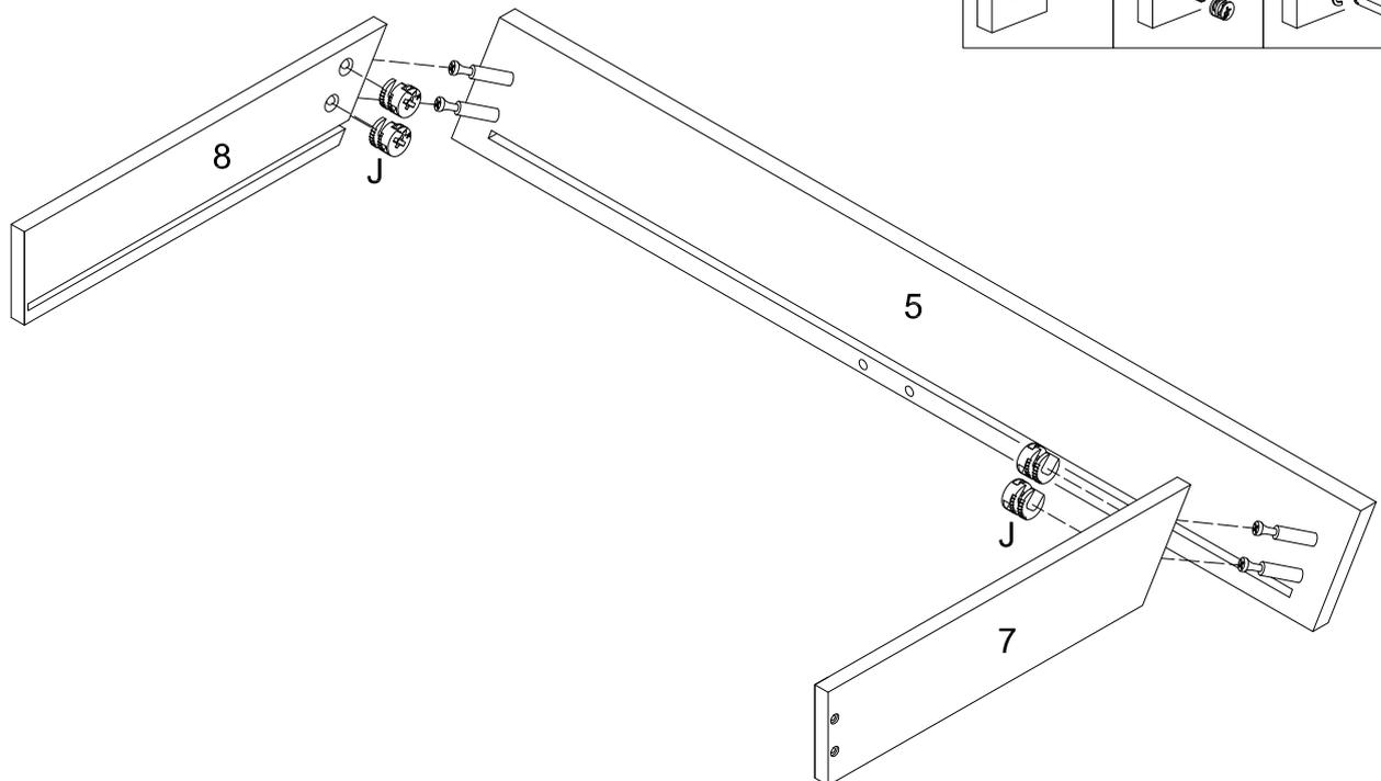
Attach the Front Panel and secure it with the Cam lock (J) for both side.
