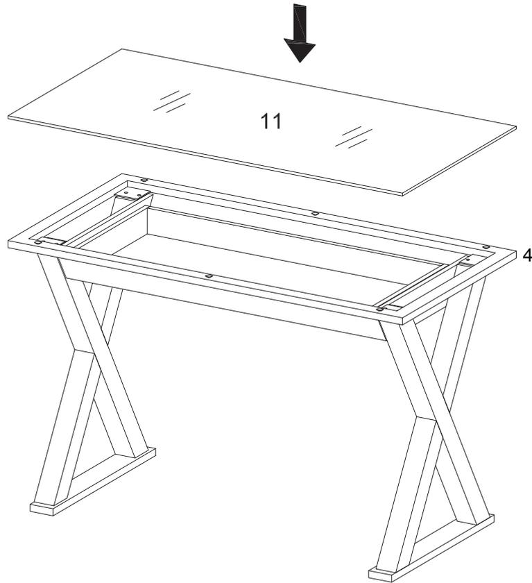
Place the Tempered Glass (11) on top of the Frame (4) and finished.
