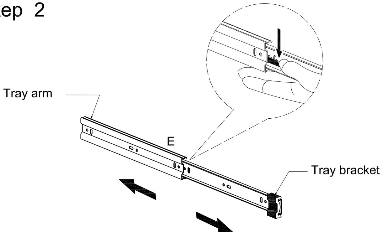
Disassemble keyboard tray slider (E) by sliding the tray arm and the tray bracket apart. Depress the small lever on the tray bracket and carefully pull the two pieces apart. Repeat this process for both keyboard tray sliders (E).
