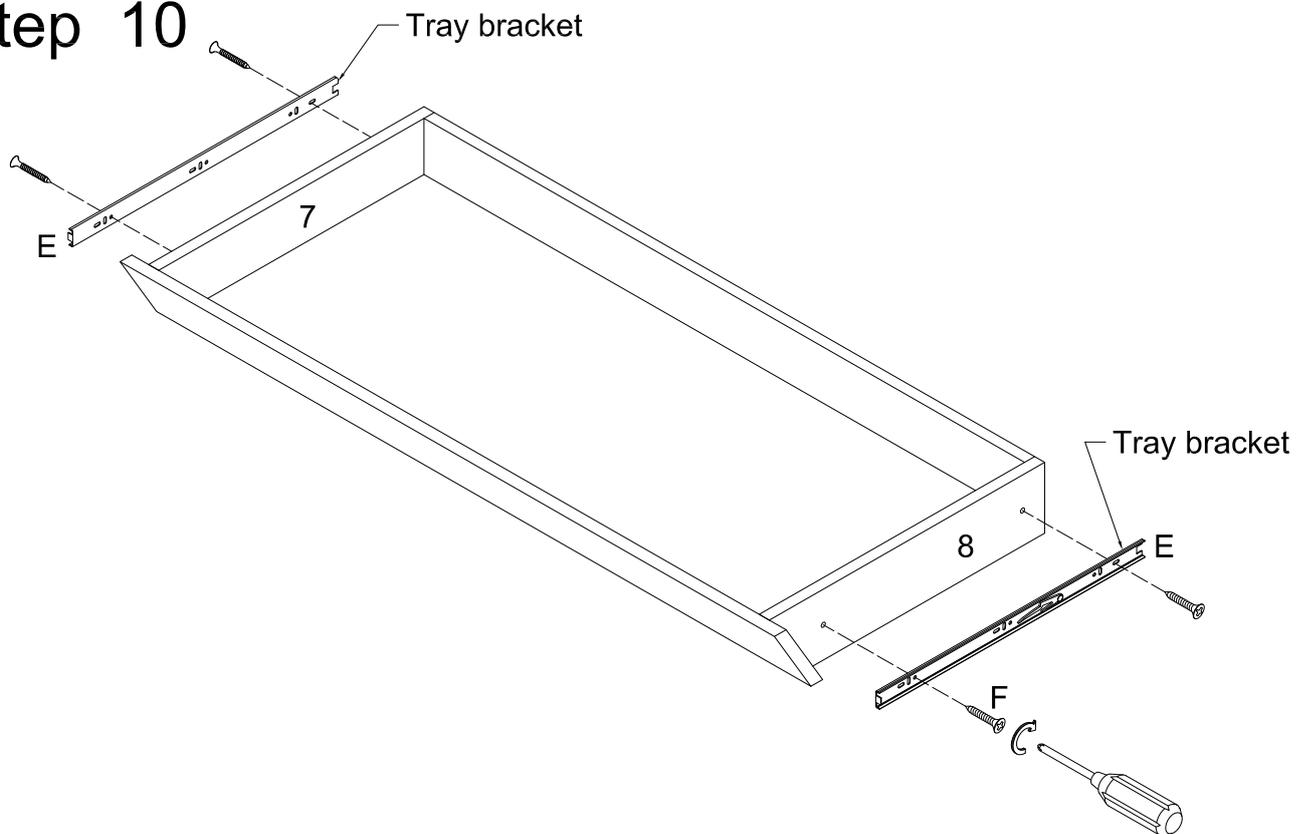
Attacher the tray bracket of keyboard tary sliders (E) on the Drawer Side Panels (7) & (8) by using Screws (F) and the Screw Driver.
