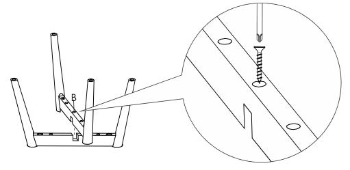
Attach part (2) to part (3) using screwdriver and srew (B).
