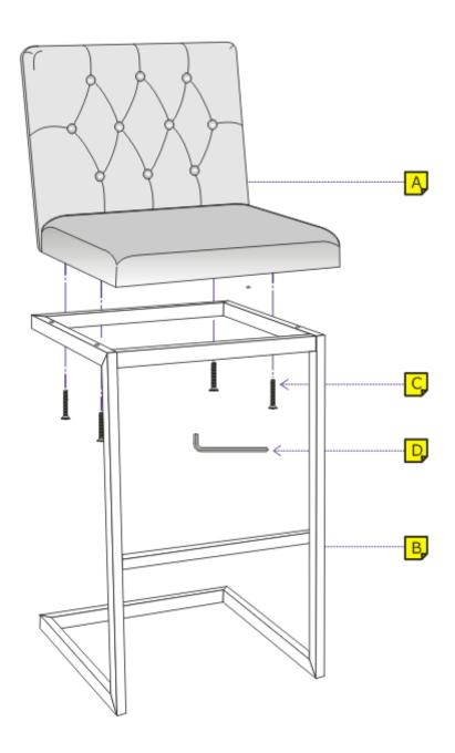
As the picture shows. Tighten the screws.
