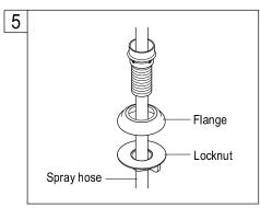
5. For model with spray head and hose, place the spray guide through the fourth hole in the sink, screw the locknut onto the shank and tighten firmly.
