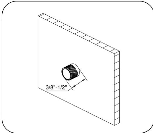
1. Shut off water supplies. Install the supply piping so that the 1/2" threaded connection protrudes approximately 1/2" beyond the finished wall.
