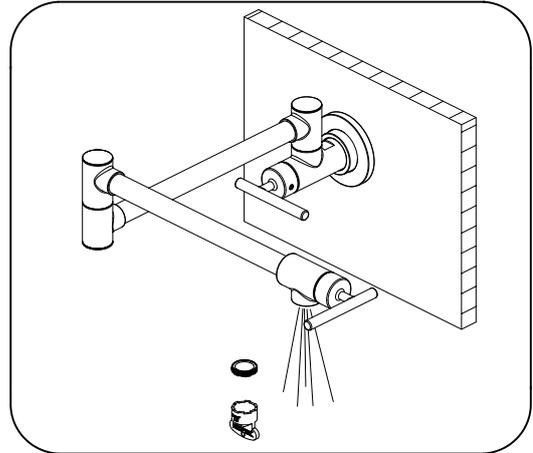
8. Turn on water supply in preparation to water test the faucet. Remove aerator with plastic wrench and turn on faucet for approximately two minutes to flush any debris from the water line. Run water into a large pan or bucket. Replace aerator and clean faucet with warm water and a soft cotton towel.
