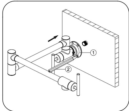
2. Install the mounting bracket (1) onto the finished wall. Screw the faucet onto the supply tubing and mark the locations for the support screws with a pencil (2).
