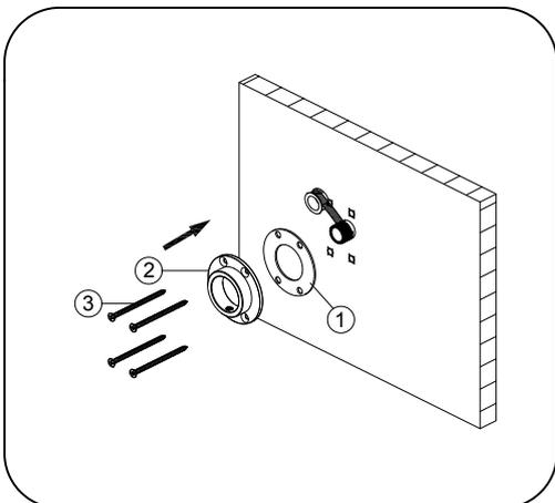
5. Wrap thread sealant tape around the threads of the supply pipe. Install the gasket (1) and the mounting bracket (2) using the 4 screws (3) provided.
