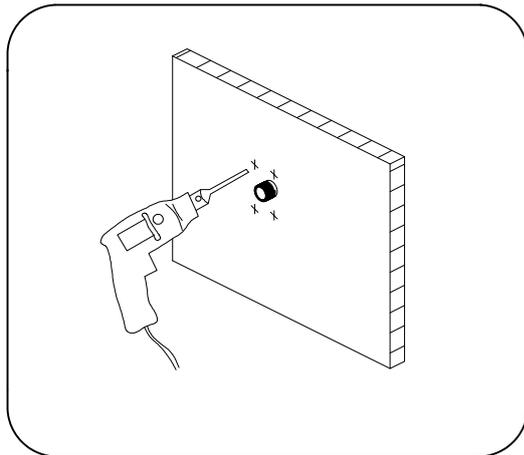
3. Remove the faucet and drill four holes on the positions marked in step 3.
