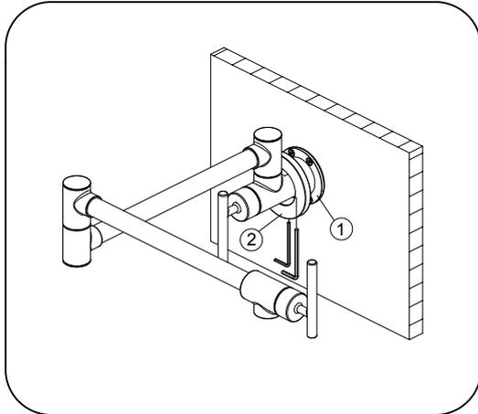
7. Tighten set screw in mounting bracket (1). Slide flange (2) over the mounting bracket and tighten set screw.
