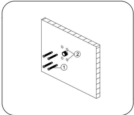
4. Insert anchors (1) into holes (2) and tap flush with wall.
