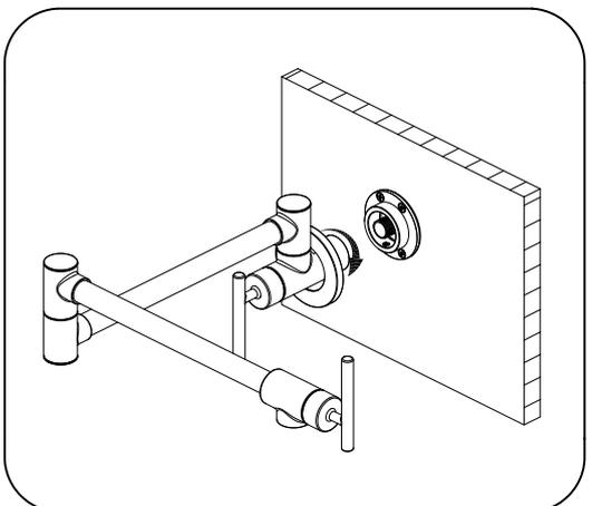
6. Place flange (1) onto the faucet as shown. Thread faucet onto pipe. Use cloth to protect finish. Tighten securely, but do not overtighten.
