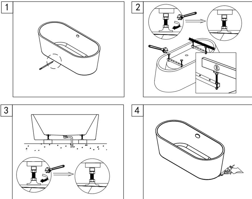
1. Move the bathtub into the desired location and mark on the floor along bathtub's bottom.
