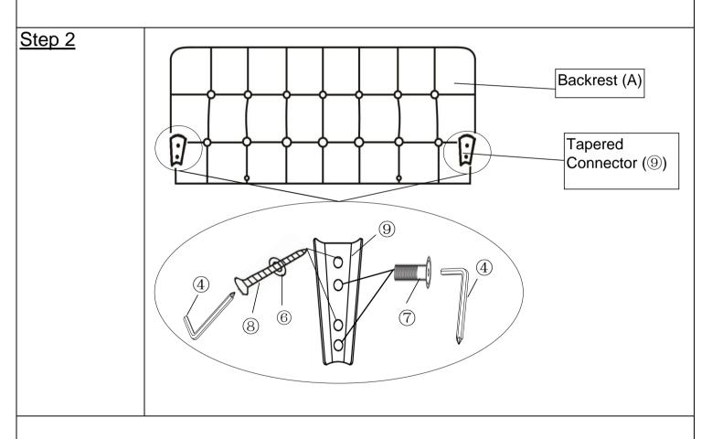
Attach Tapered Connectors(9) onto both sides of Backrest(A) using Bolts(7), Screws(8) and Washers(6) with Allen Key(4) as indicated in the diagram above.
