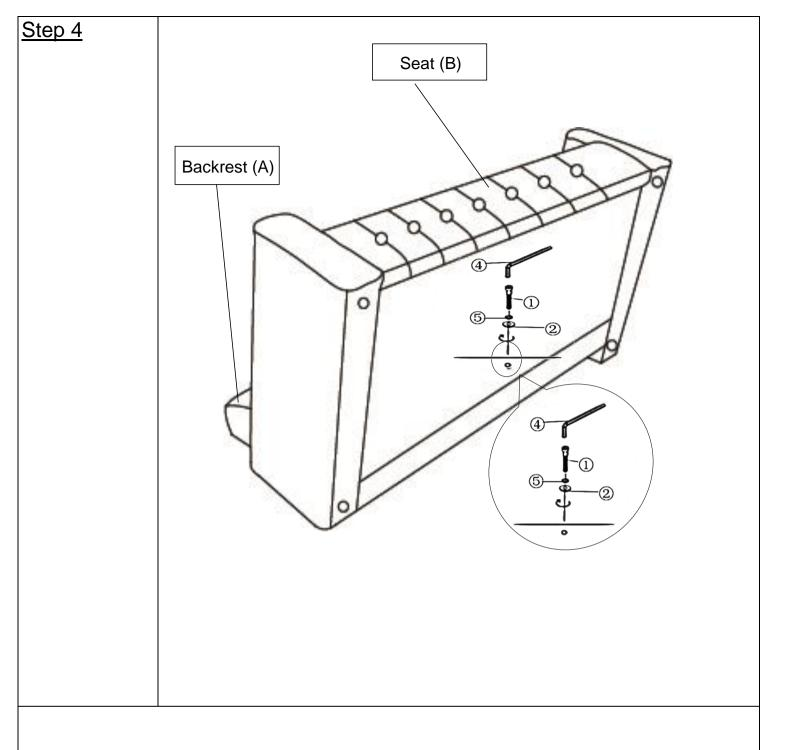
Attach Seat(B) to Backrest(A) using Bolts(1), Spring Washers(5) and Washers(2) with Allen Key(4) as pictured above.
