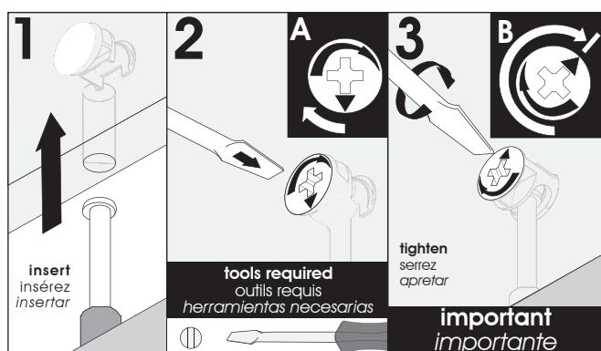
**Make sure to properly tighten each cam to ensure furniture solidity. Otherwise, parts could be damaged or the user could be injured.**
