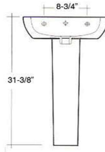
Dimensions of fixture are nominal and may vary within the range of tolerances established by ASME Standard A112.19.2-2008. Dimensions and specifications subject to change without notice.
